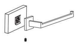
Slide body assembly onto mounting bracket.
