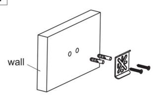
Install mounting bracket to the wall with screws(supplied) and anchors(if applicable).
