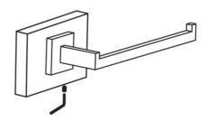
Tighten set screw with allen key (supplied).
